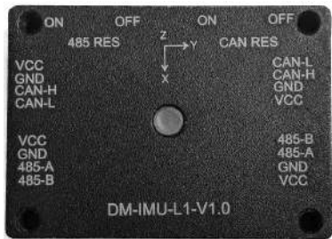
IMU模块：DM-IMU-L1
